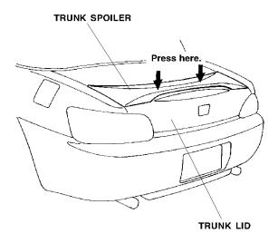
Slowly remove the trunk spoiler from the trunk lid. Check that the marking washers stay attached to the trunk lid.
